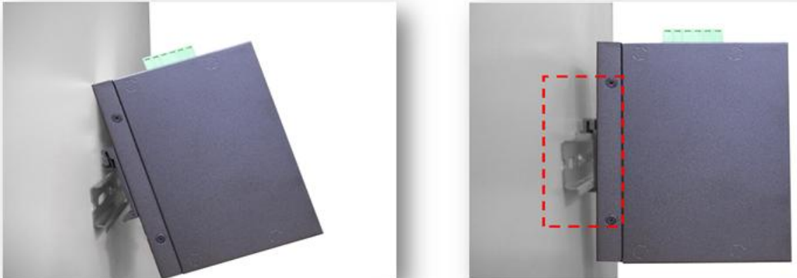
Figure 3.2 - Insert the Switch on the DIN- Rail
